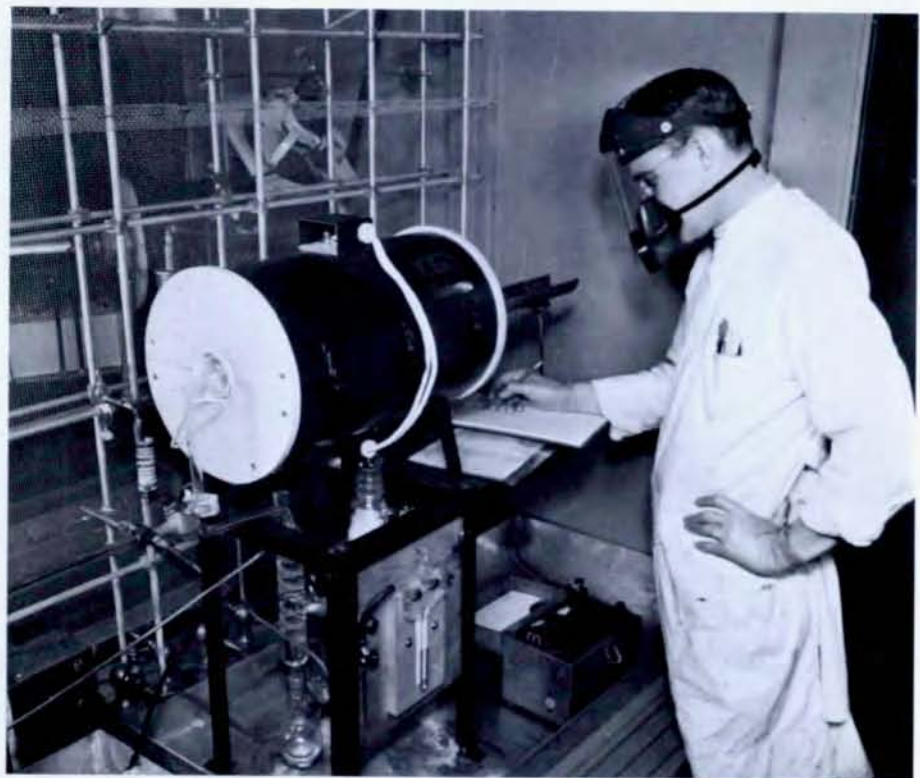
The hydrofluorination of plutonium. The upper photograph shows the chemical hoods in D Building used for this process, which converted the oxide to the tetrafluoride. Four furnace controllers are at the top of the panel with one controller open showing the temperature program cut into its rotating disc. Note the bucket of calcium oxide to be used for treatment of hydrogen fluoride burns. The lower photograph shows one of the hydrofluorination furnaces inside the hood.
